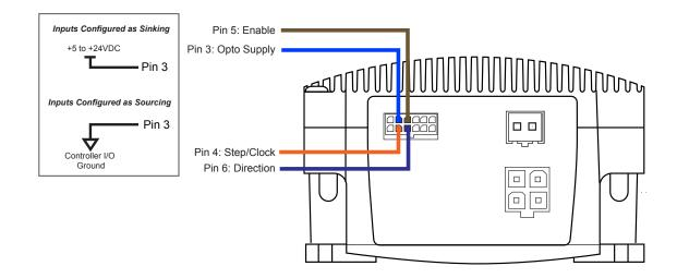
Figure 2.4.1: Isolated Logic Pins and Connections
